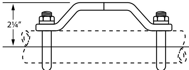
Type "U" base for pipe mounting is designed to provide secure, non-slip mounting of the bus support assembly to pipe. Standard base fits pipe sized 1-1/4" S.P.S. Bases available for other pipe sizes. Mounting holes 45° to tubing.
